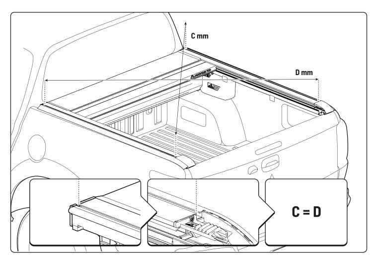
• Ensure the cross measurements are identical.
