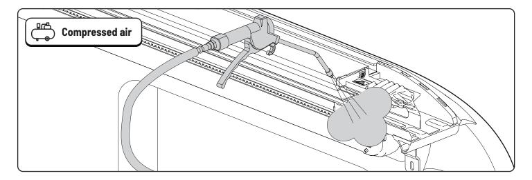
Remove dirt and debris using compressed air.
